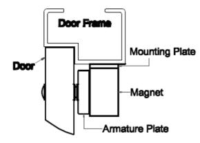
**Note:** To make the armature plate adjust its proper position to the magnet automatically, do not fix the armature plate too tightly and make the rubber washer more flexible.
