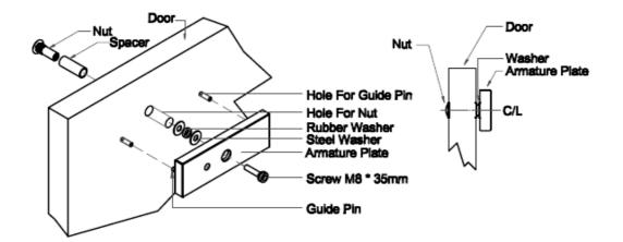
Typical Installation of the electromagnetic lock:
