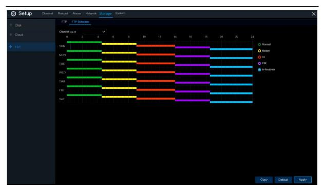
FTP Schedule: Need to configure the plan to perform FTP file uploading.
