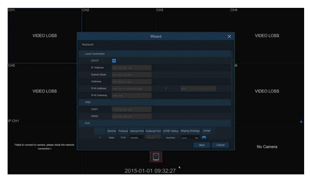
If you connect to a router that allows you to use DHCP, please check the **DHCP** box. The router will automatically assign all the network parameters for your DVR. Unless the network is manually addressed as the parameters below:
