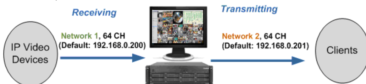
GV-VMSH V6 + 2 Network Cards assigned on different networks
