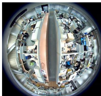
Figure 5-10 Once the image of GV-FE2301 / 4301 is aligned, all four edges of the image will be cropped slightly.
