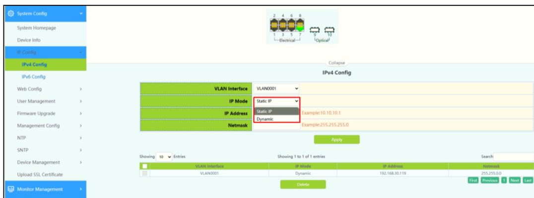
2. In IP Mode, select **Static IP** to change an IP address or click **Dynamic** to allow DHCP to assign a dynamic IP address. Click **Apply**.
