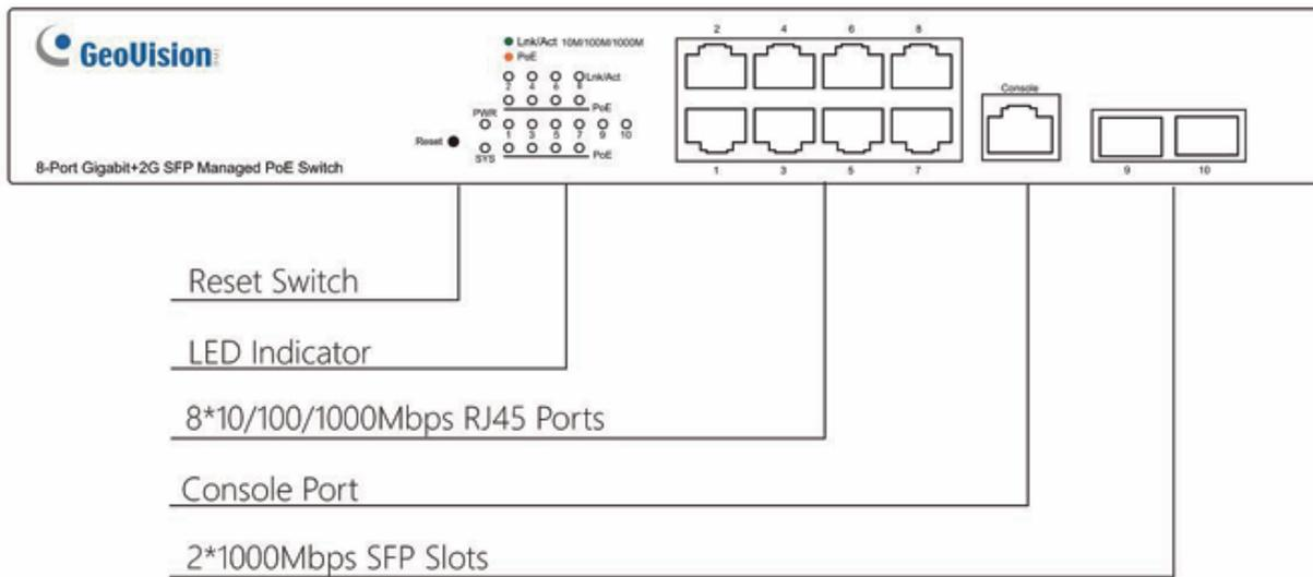
**IMPORTANT:** The Console port is used to connect to the serial port of a computer or other terminal device for debugging only.
