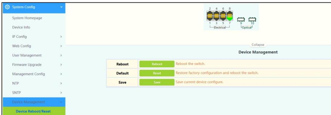
**Note:** After loading default by pressing the Reset button or from the Web interface, you may need to configure IP address and Password again.
