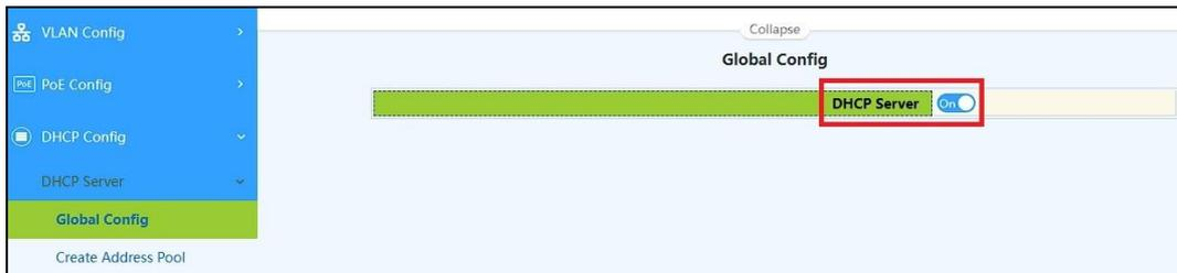
3. To create an address pool, select **DHCP Config > DHCP Server > Create Address Pool**. Here, we create an address pool called "1" as an example.
